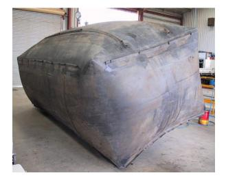
Road train trailer lined with a flexi tank enable the trailer to cart both solids and liquids.
